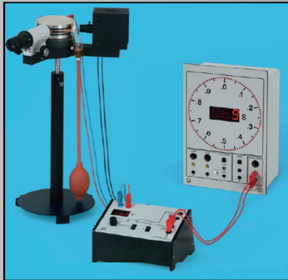
Determining the electrical charge of the electron after Millikan
